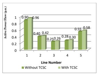
**Fig. 7** Comparision of Power flow with and without TCSC for a 5 Bus System-TCSC Location Line 7 ALPHA=152.3273 $^{\circ}$
