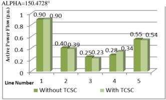
Fig.6 Comparision Of Power Flow With And Without Tcsc For A 5 Bus System-Tcsc Location Line 4
