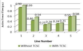
Fig. 4 Comparision of power with and without TCSC for a 5 bus system-TCSC Location Line 2
