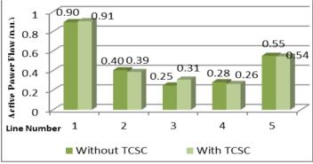
**Fig. 5** Comparison of Power Flow with and without TCSC for a Bus System –TCSC Location line 3
